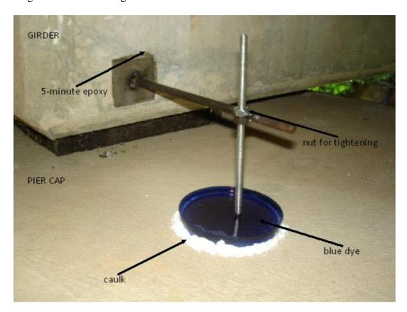
Figure 3.4.2: Photo of an in-place wax plate at the Bartow County bridges (StructBAR1, interior bent)
