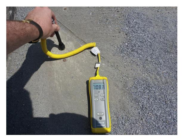
Figure 3.4.7: Deck surface temperature reading being taken with thermocouple
