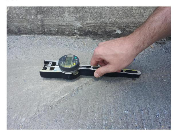
Figure 3.4.6: DEMEC reading
